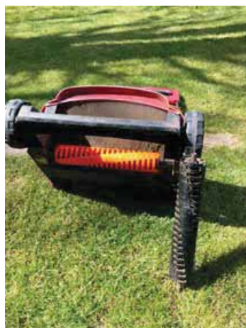
This lawn scarifier needed a new drum because the old one was worn out, our repairers helped by fitting it.
