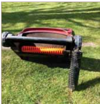
This lawn scarifier needed a new drum, our repairers helped by fitting it.
