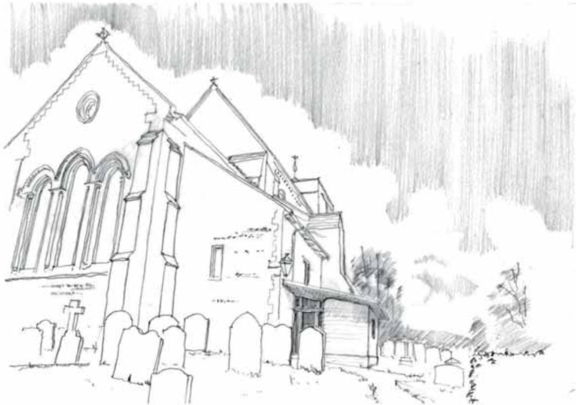
View showing the proposed new accessible entrance to the church, which will include an accessible WC and small lobby space to accommodate buggies and turning space for wheelchairs. New glazed doors provide plenty of daylight to help create a welcoming entrance. Materials could include stone, and a zinc roof which can be used on shallow pitch roofs.
