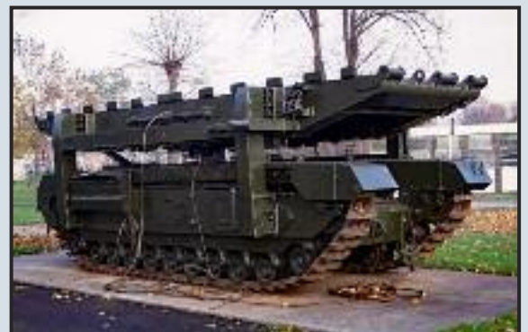
'Hobart's Funnies' was a name given to specialised WWII military vehicles, such as this Churchill tank with bridge layer (Murgatroyd49, Wikimedia Commons)
